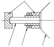
PUSHROD LOCKNUTS **THRUSTER**
